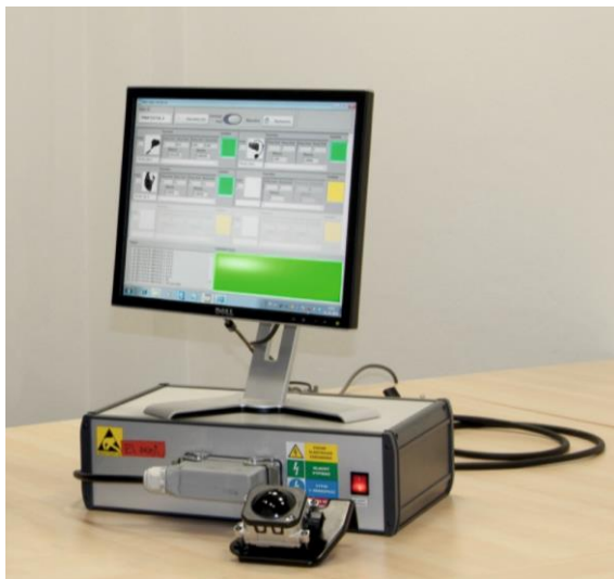
Installation for testing automotive cable assemblies
